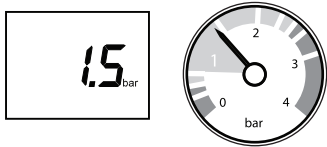
Fig.51 Restore water pressure
