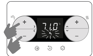
second press set DHW setpoint value in steps of 0.5 °C
