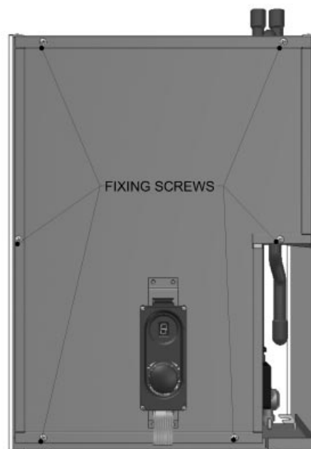
Fig. 26. Combustion Case Panels
