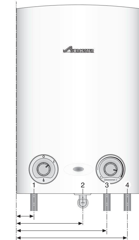
Fig. 19 Pipe work dimensions
