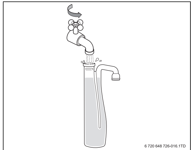
Fig. 78 Filling the condensate trap with water
